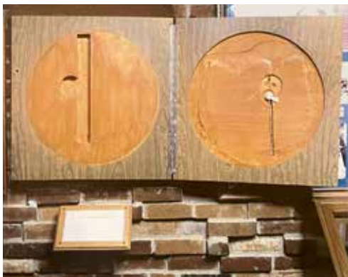
Replica of Great Seal opened to show resonant cavity and microphone placement, United States Collection National Cryptologic Museum
